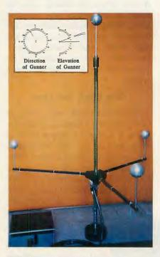
Bullet Direction Indicator uses four spherical sensing heads to compute location of sniper from shock wave produced by passing projectile. Bullet origin is given by an azimuth indicator and elevation scale. Photo: courtesy GD Associates
